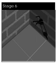
6. Seal the perimeter with a suitable exterior grade sealant before fixing tile skirts.
