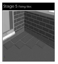
5.Once the boards are securely fixed and the adhesive sufficiently cured tiling can begin. Fix tiles using a suitable exterior grade cement based flexible adhesive. Finish with a suitable exterior grade flexible grout. Avoid grouting the external perimeter as this should be sealed using a suitable sealant later
