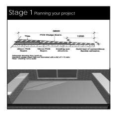
1.PCS wedge boards are used in conjunction with PCS thermal construction boards which are used to raise the wedge boards maintaining falls over any distance. It will be necessary to pre plan the setting out of the floor as you may require different thicknesses of boards for the raising course.
