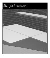
3. Prime floor using a suitable exterior grade primer. Fix boards using an exterior grade flexible cement based tile adhesive applied with large notched trowel to form a level base. Boards must be pressed firmly into adhesive whilst the adhesive is still tacky. Use a straight edge to ensure falls are maintained
